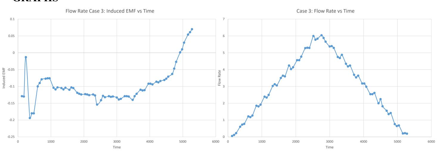
These graphs show induced EMF(left) vs time compared to the change in flow rate vs time(right).
