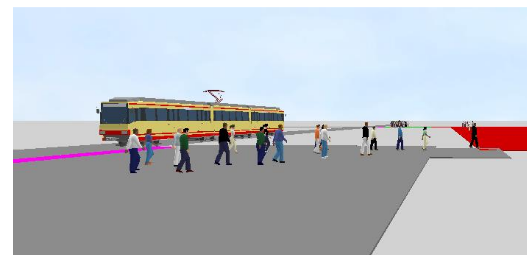
VISSIM Model showing movement off one mode of transportation and onto another.
