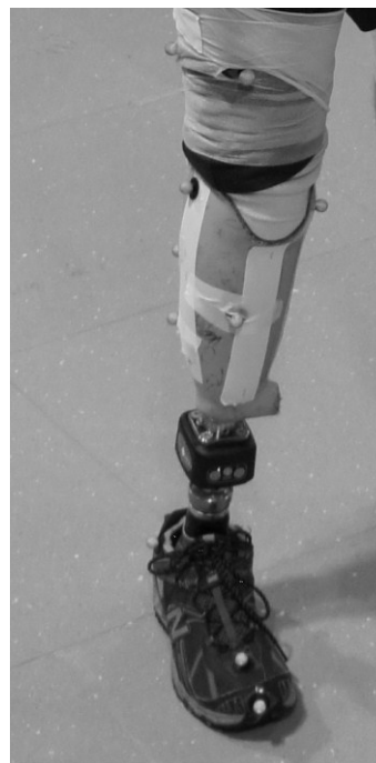
Figure 35: Prosthesis with iPecs sensor below the socket
