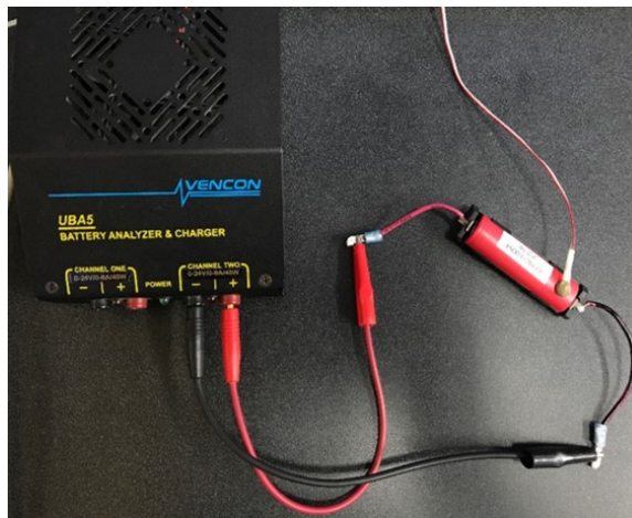
Figure 3.1 UBA5 Battery Tester is Testing an NCR-18650 Battery Cell.
