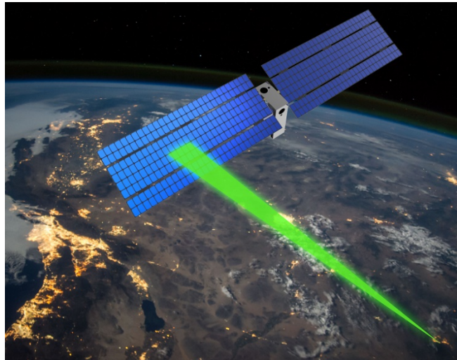
Figure 1: Lasers from the ground or space will interact with solar panels of the derelict spacecraft to power and it as part of space traffic management activities.
