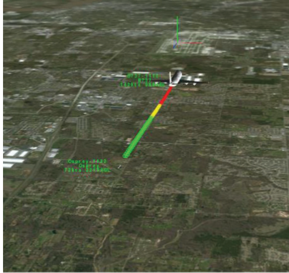
Figure 2.1: Wake vortex rings behind the leader aircraft.
