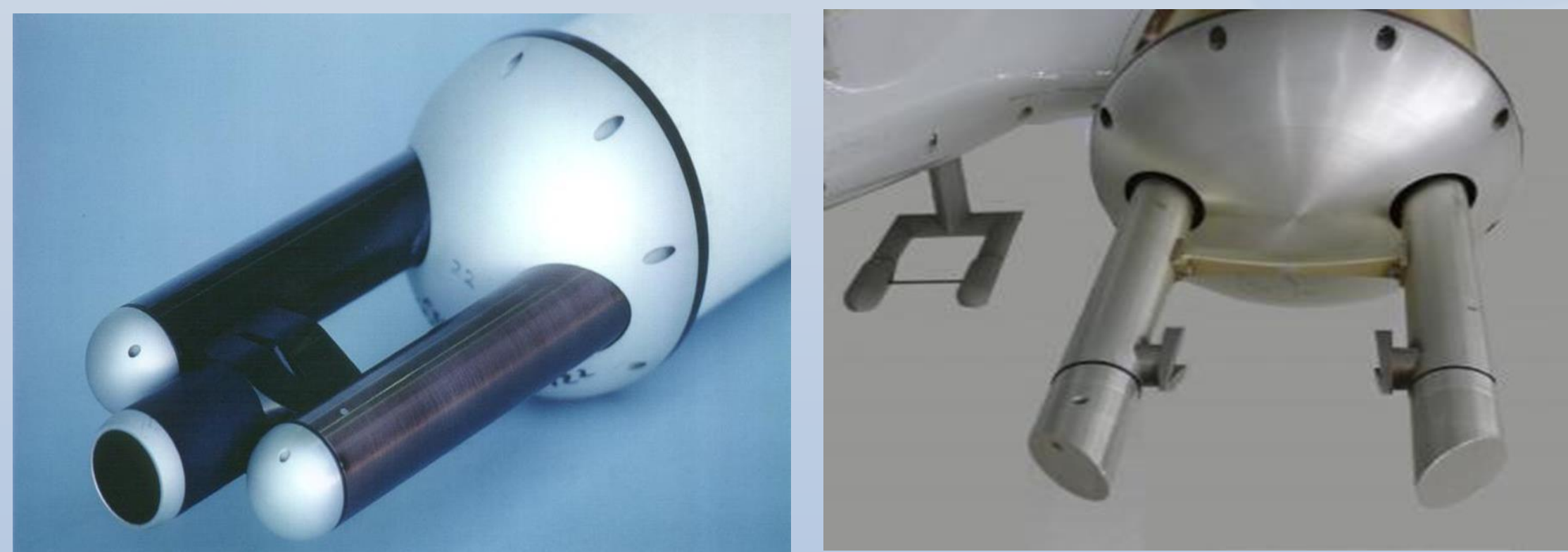
Fig. 1 The FSSP and 2-DC instruments package (courtesy of NASA Airborne Science Program)
