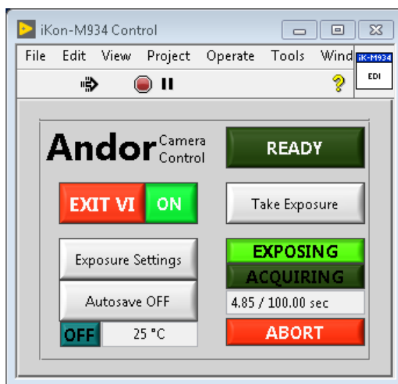
Figure 4.16: The Andor camera control widget is very minimal. The user can change the exposure settings, turn on cooling or autosave, and take exposures. In this image, the widget is currently monitoring an exposure.
