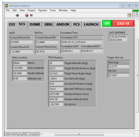
Figure 4.20: The cluster widget allows the user to check on all of the running subsystems from one place.
