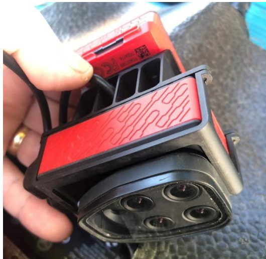
Figure 1. Parrot Sequoia Multispectral Camera.
