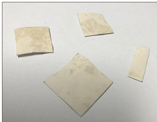
Figure 25. a) PVDF/PZT 0-3 Composite after it is cut.
