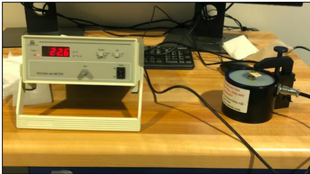
Figure 38. d33 measurement of the polarized sample.
