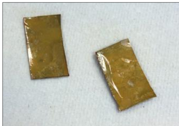
Figure 31. Sample coated with photoresist.
