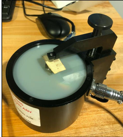
Figure 39. Device used to set mN force to the sample.
