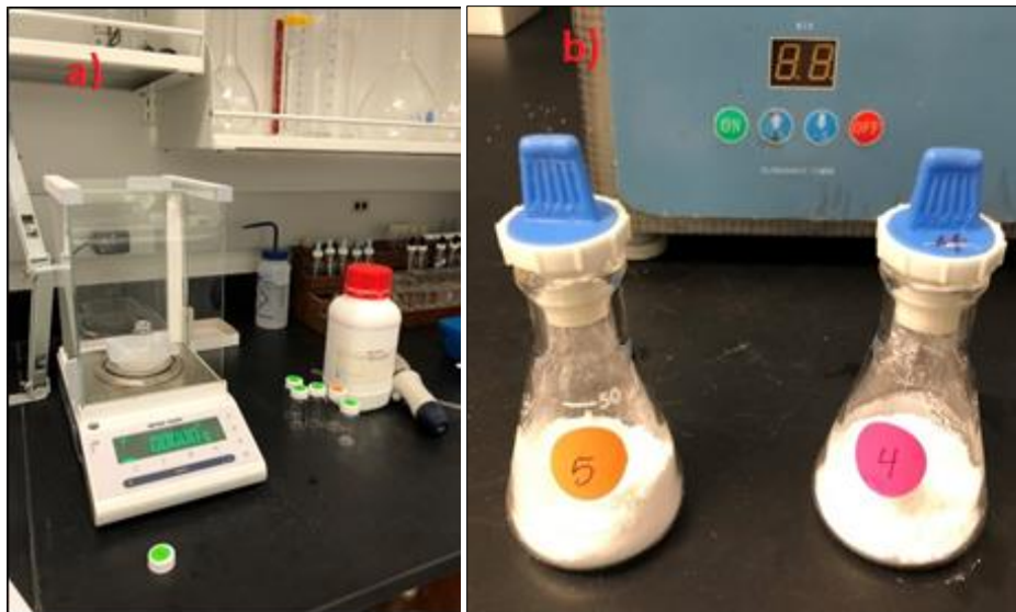
Figure 20. a) Weighing PVDF using a digital balance, b) Measured PVDF powder.
