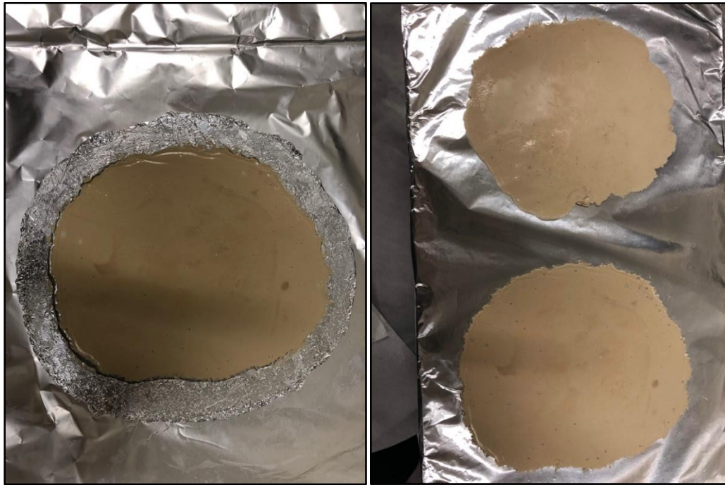
Figure 24. PVDF/PZT sample cooled to room temperature and let dry for a day to get the flat round composite.
