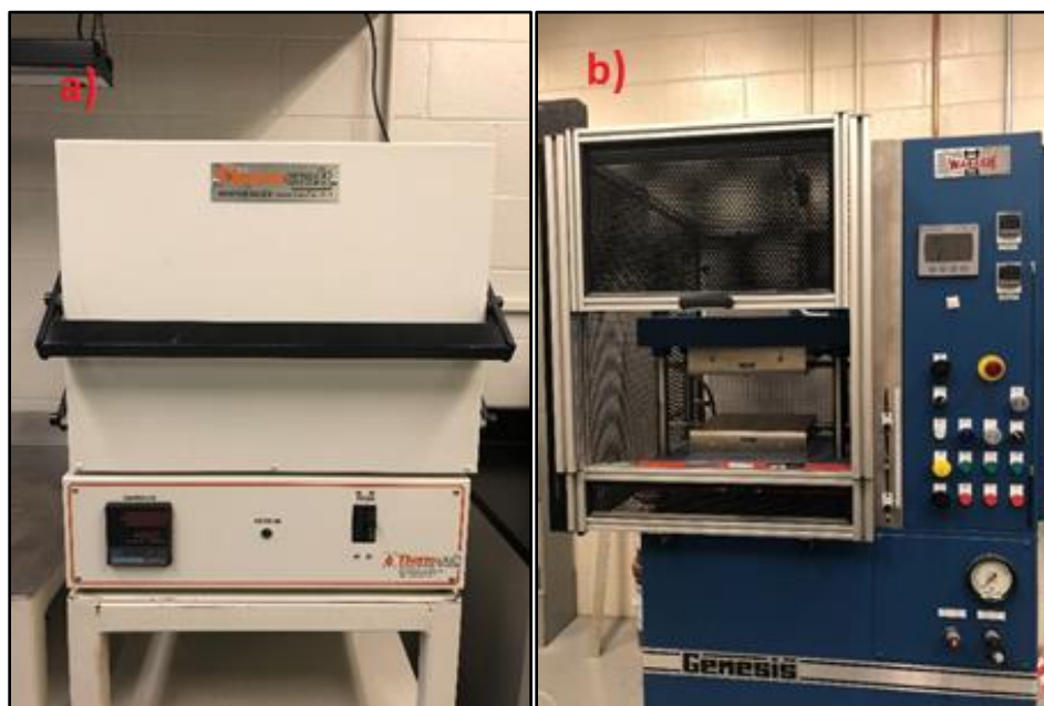
Figure 23. a) Oven heating of the solution to evaporate DMSO b) Hot-pressing the dried mass.
