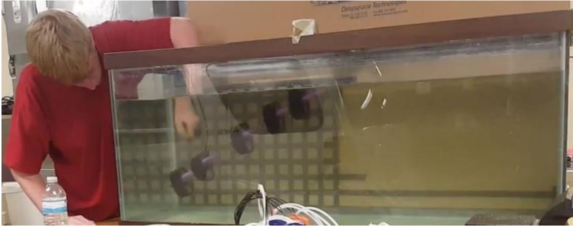
Figure 28 Composite Image Illustrating Inverse Zimmerman Planform featuring an Annular Wing's Glide Path
