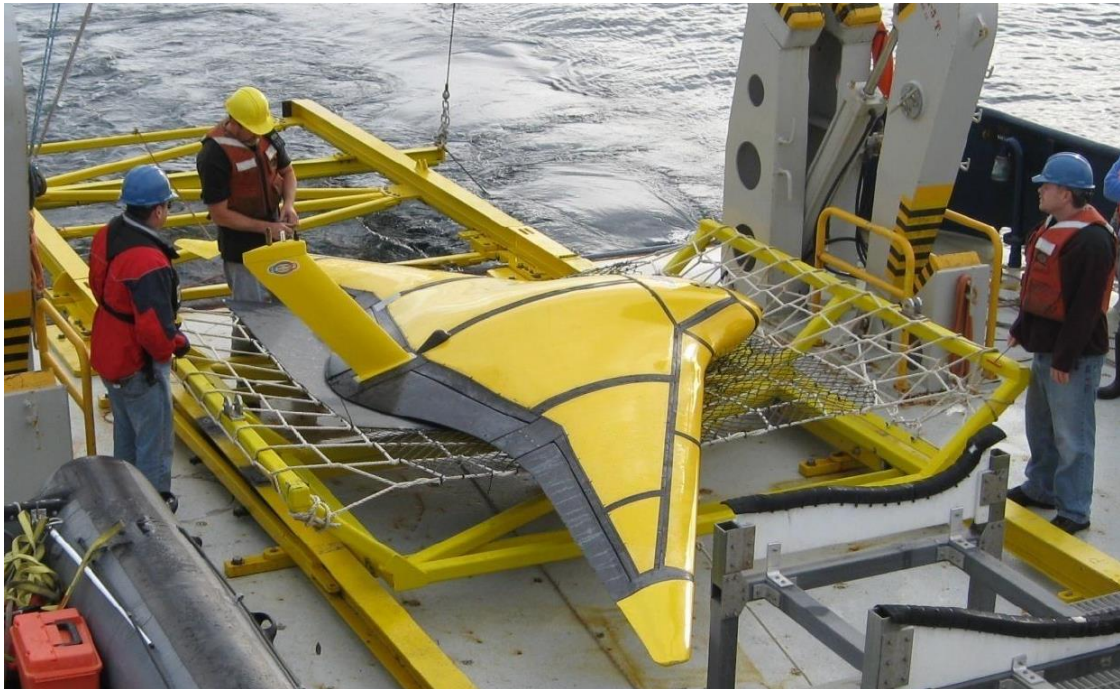
Figure 24: A Flying Wing Type Seaglider Retrieved from [30]
