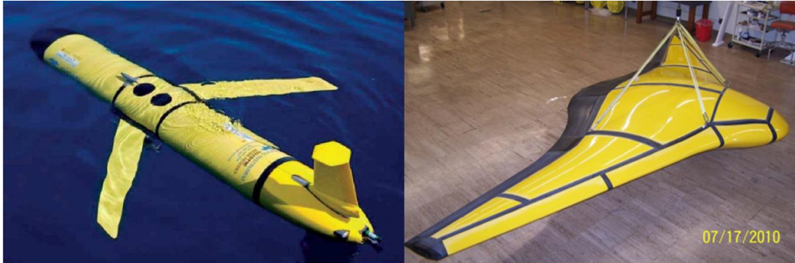
Figure 2: Legacy Type Glider (Slocum Seaglider Left) [2] and a Flying Wing Type Glider (Liberdade XRay1 Seaglider Right) [3]
