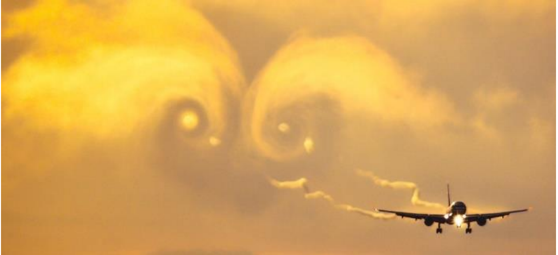
Figure 26: An Example of an Aircraft Producing Wingtip Vortices Produced by an Aircraft Retrieved from [78]
