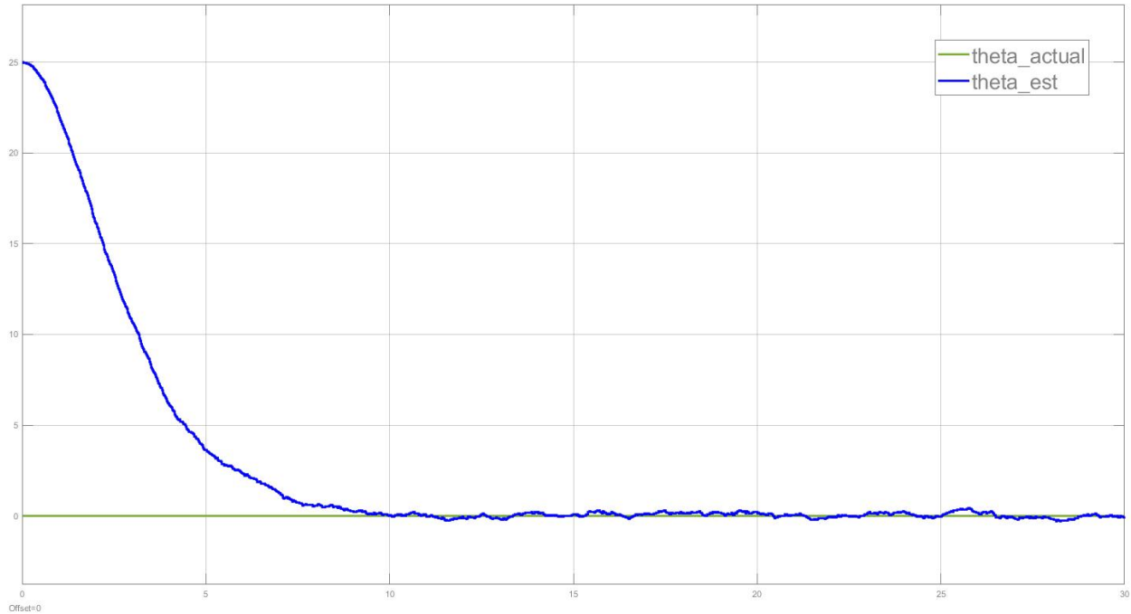
Figure 5-32: Initialization Error - Airspeed Aided Inertial Attitude EKF
