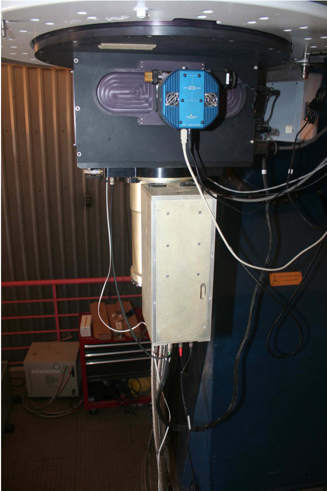
Figure 4. Tailpiece of the SARA-KP telescope in 2016 July, showing the acquisition and guiding box above the ARC CCD camera. The covers for the guider track are visible on either side of the octagonal box housing the heat exchangers for the guide camera's cooling assembly.
