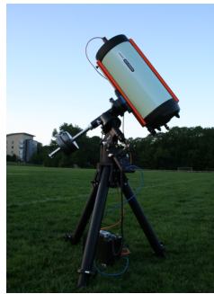
Figure 1. OSCOM telescope system for small satellite and debris photometry deployed in Needham, MA, USA. Used with permission from Gasdia et al. [14] © 2016 AMOS Conference.
