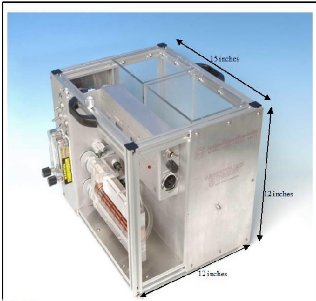
Figure 1: DLM with shell and tube heat exchanger cartridge inserted. The on/off switch is located on the right side of the DLM, digital display for temperature and pressure readings are just above cartridge. The shell and tube cartridge plugs into the main module with standardized ports for quick swapping of one cartridge with another.
