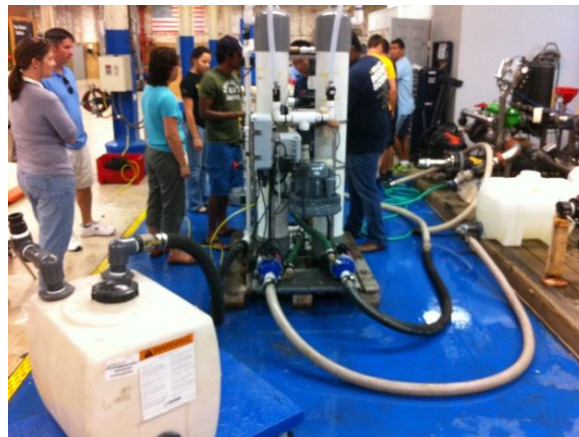
Figure 3 Wet Table Testing with Fine Red Clay Dust
