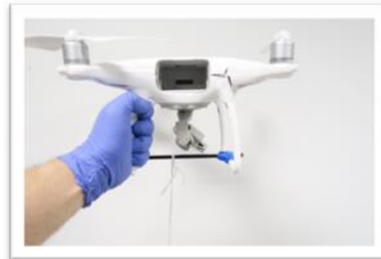
(b) UAV load carrying (Image shows a DJI Phantom, where a rod of plastic has been taped spanning the legs. A string can be seen hanging down, which would have held the payload).
