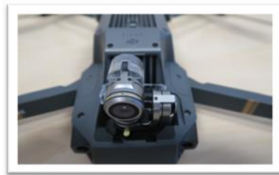
(a) UAV with a camera (HD camera fitted to a DJI Mavic Pro).
