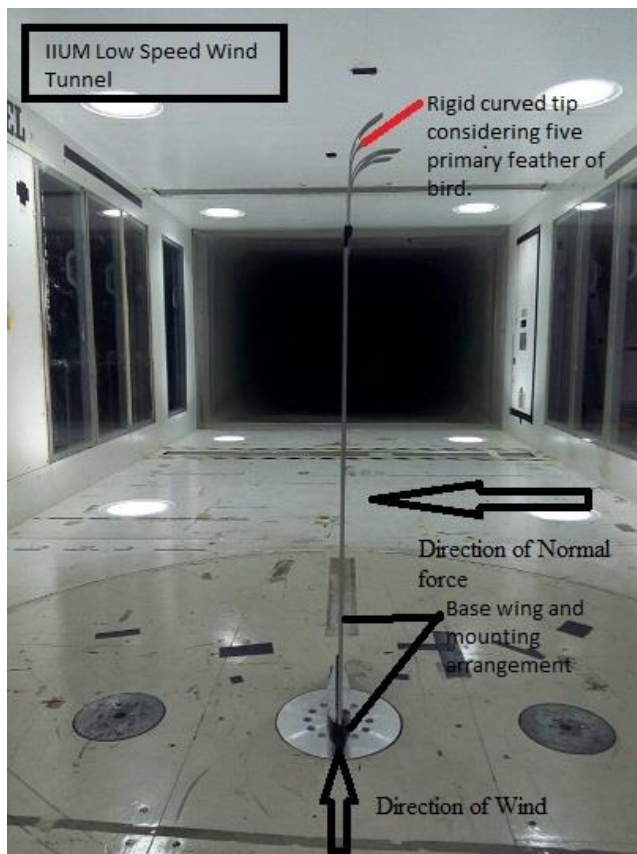
Figure 6. Flat plate wing (Base wing) with rigid curved wing tips of 2mm thickness inside the IIUM wind tunnel.
