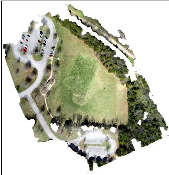
Figure 10. The output of the PhotoScan software combining all 29 images.
