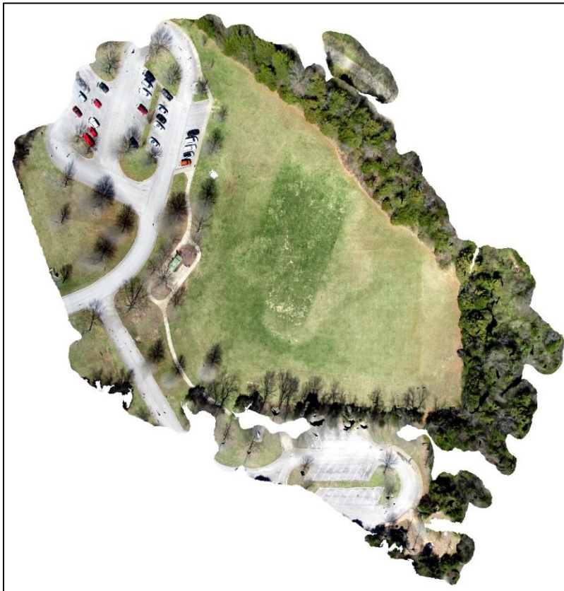
Figure 9. The output of the PhotoModeler Scanner software combining all 29 images.
