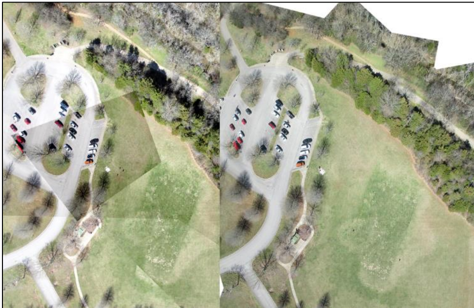
Figure 5. Comparison of individual georectified images to a georectified composite section.
