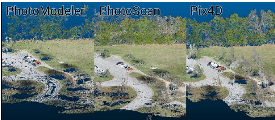
Figure 17. A look at the bare trees in the point clouds, with Pix4D doing the best job of representing the true heights of the bare trees.
