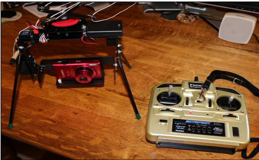
Figure 2. Remotely Controlled Camera Rig Holding the Canon ELPH PowerShot 130IS.
