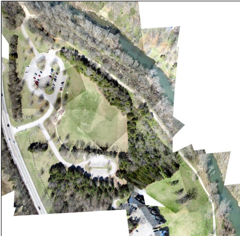
Figure 4. A collection of images individually georectified and displayed in ArcGIS.
