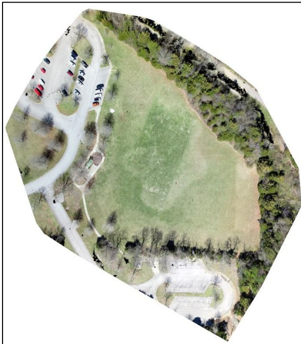
Figure 11. The output of the Pix4D software combining all 29 images.
