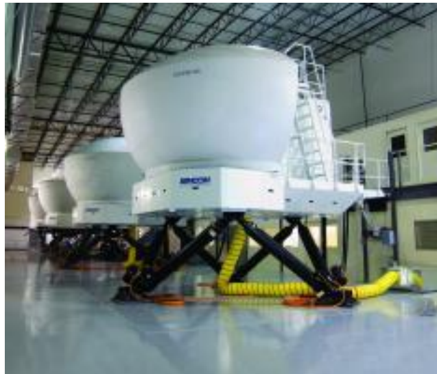
Figure 3. Full Motion Level 3 / 4 Flight Simulators. BART International – Simulators at SimCom Training Center. (Retrieved from http://www.bartintl.com/content/simcom-pks-sim-bay3909rsjpg Reprinted with permission.)
