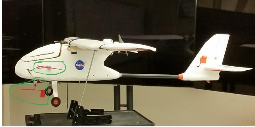
FIG.3: Display a plane with an AOA and SA vanes connected to a Hall-Effect sensor.
