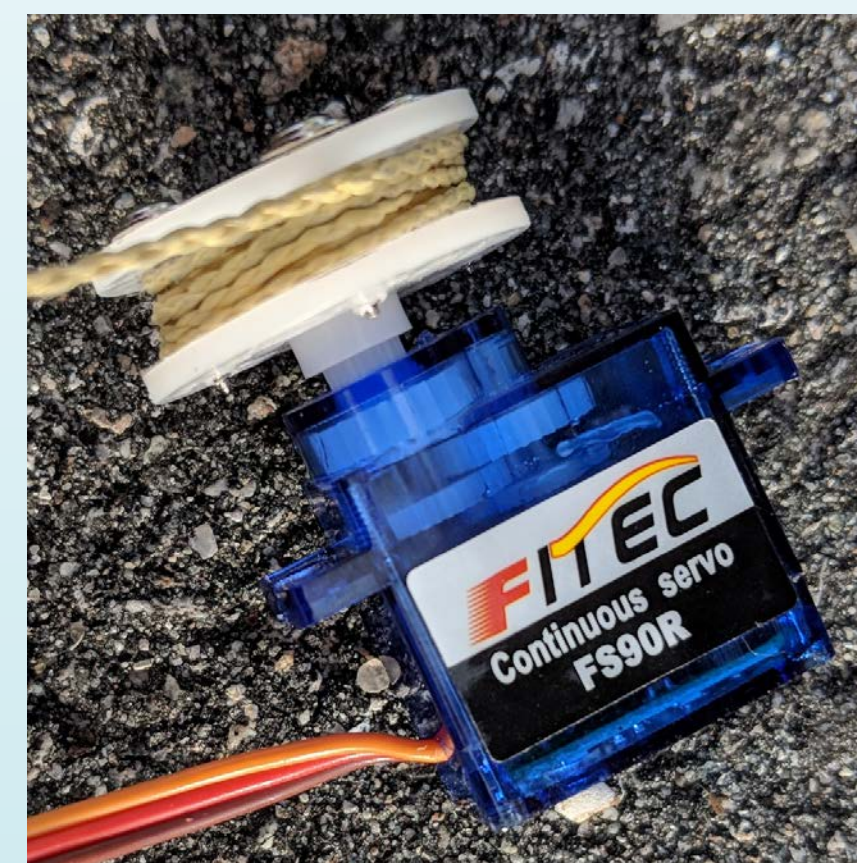
Above: Servo and attachment that controls the linear slide. Right: Fully extended linear slide.
