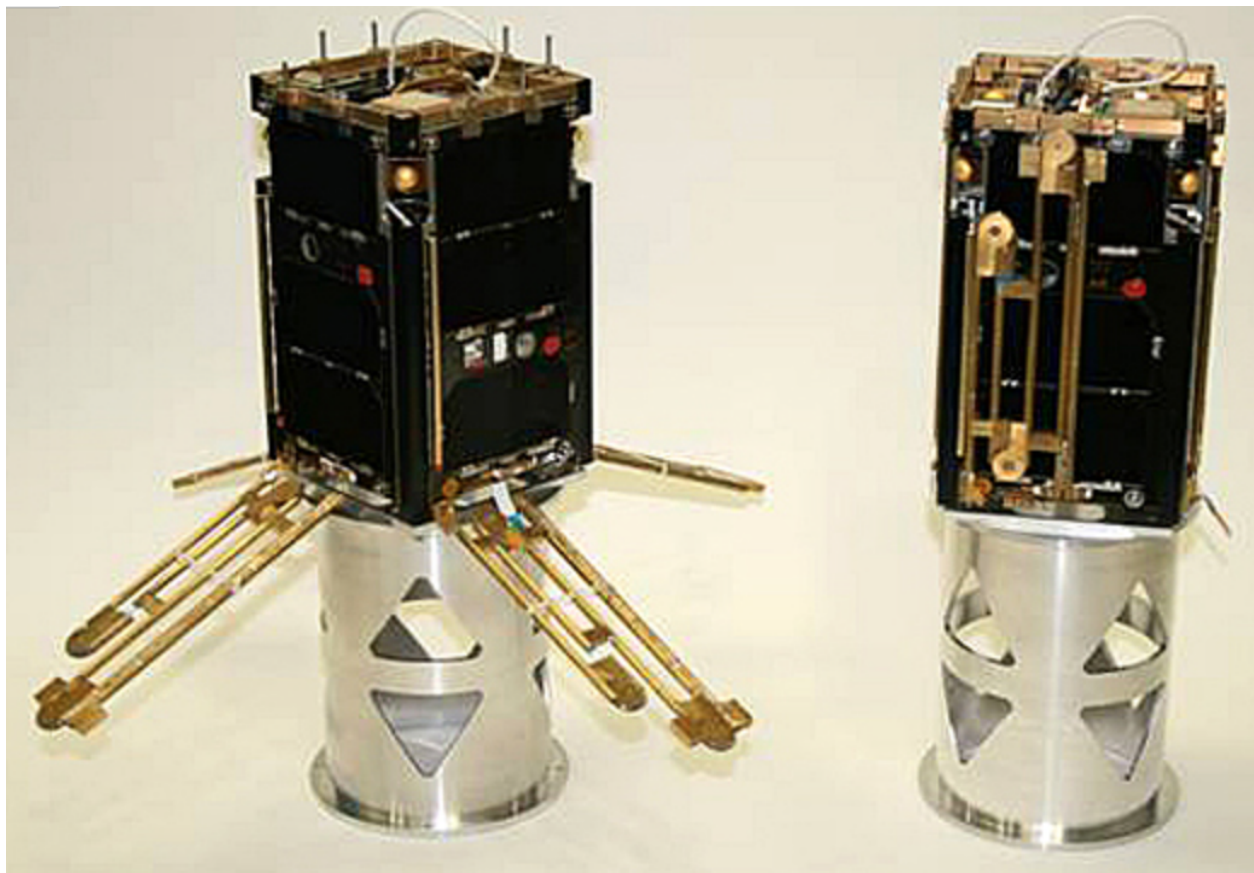
Figure 1.6: The two identical 1.5U DICE CubeSats, Farkle (DICE-F) and Yatzee (DICE-Y) [Fish et al., 2012].
