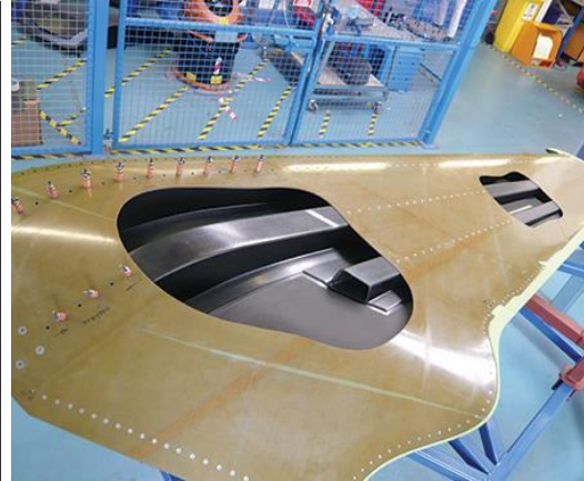
(b) GKN design with co-cured upper skin and waffle stiffener ("GKN Leads "STeM" Program to Successful Conclusion")
