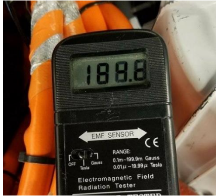
Figure 69: EMI Reading on Three Phase Cables to Motors
