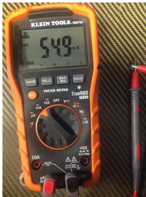
D 6: Verified Parasitic Current Draw from 12v battery
