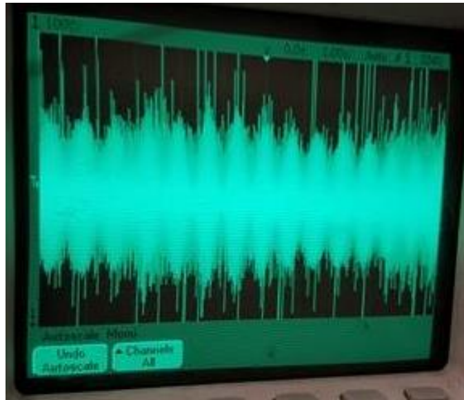
Figure 63: Voltage Ripple on 12v system before mitigation
