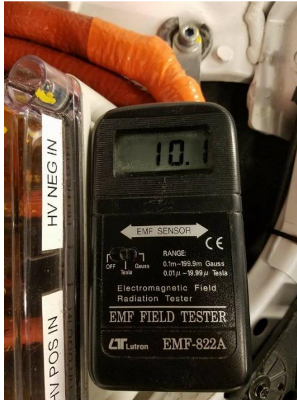
Figure 67: EMI Reading Across the DC Lines
