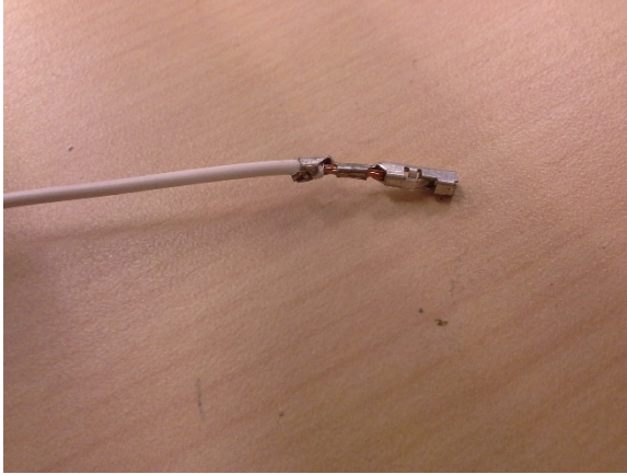
Figure 56: Bad Crimp w/ Insulation Crushed
