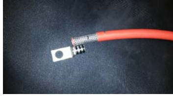
Figure 92: HV Cable step 2
