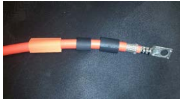
Figure 95: HV Cable step 5
