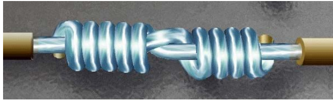
Figure 17: Completed Wrap for Western Union
