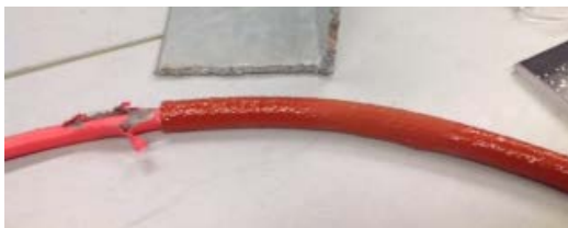
Figure 67: HV Cable Sleeving Test
