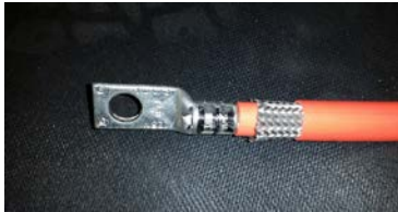
Figure 94: HV Cable step 4
