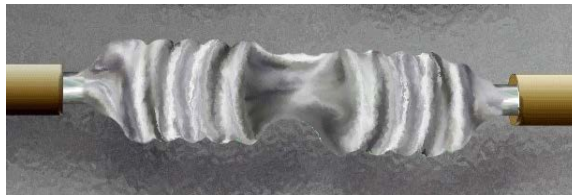
Figure 18: Soldered Western Union
