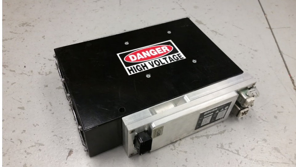
Figure 4: BRUSA HV Charger
