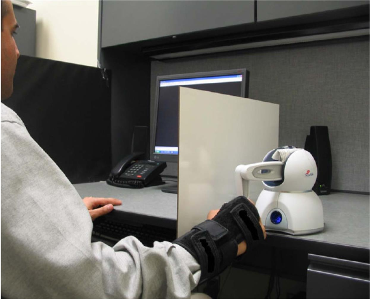
Figure 19 - Experimental Setup with PHANToM™ Omni [32]
