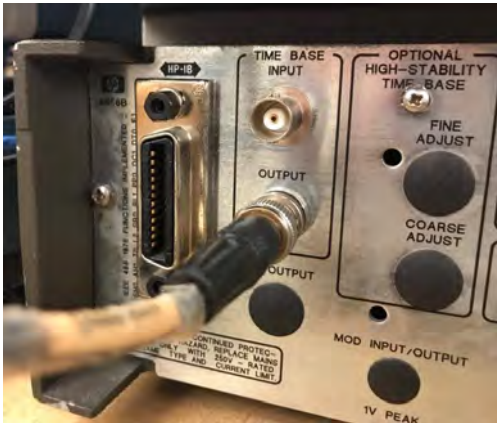
(a) Back of signal generator showing the time base output connection
