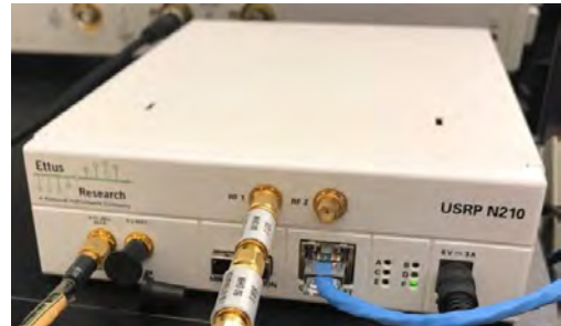
(b) Front of the Ettus N210 showing the reference in port
