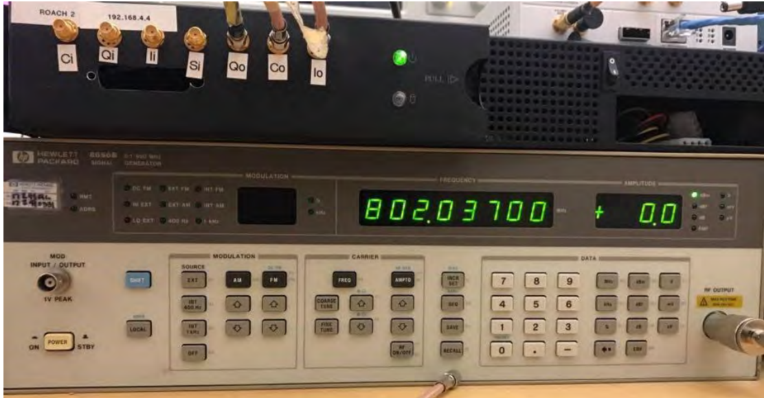
Figure 4.2: Signal Generator configurations and ROACH input/output ports.
