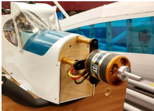
Figure 2.7 AXi 5345/18HD mounted on Rascal
