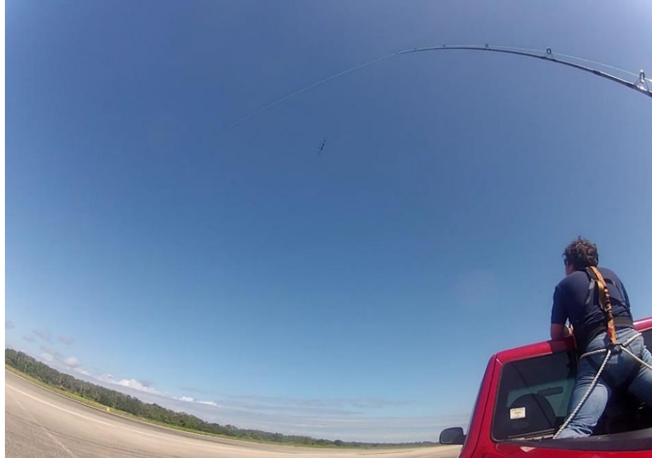
Figure 44 Pilot harnessed in a truck bed with the glider cabled to a fishing pole (taken at SLF)
