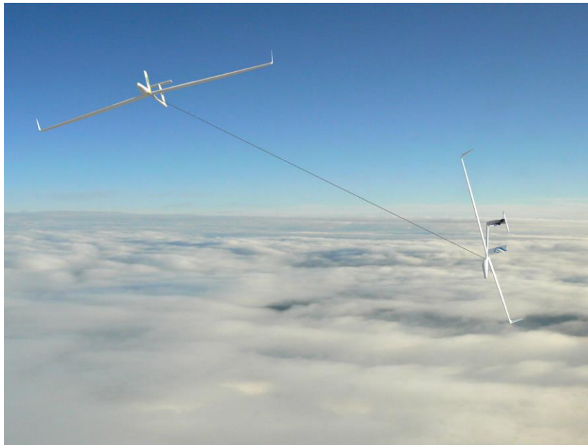
Figure 1 Dual-aircraft platform configuration (Engblom W. A., et al., 2016)
