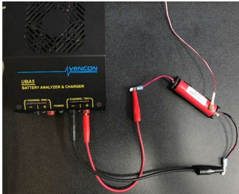
Figure 4.1 Single Cell Test Setup with the Vencon UBA5 Battery Analyzer & Charger.
