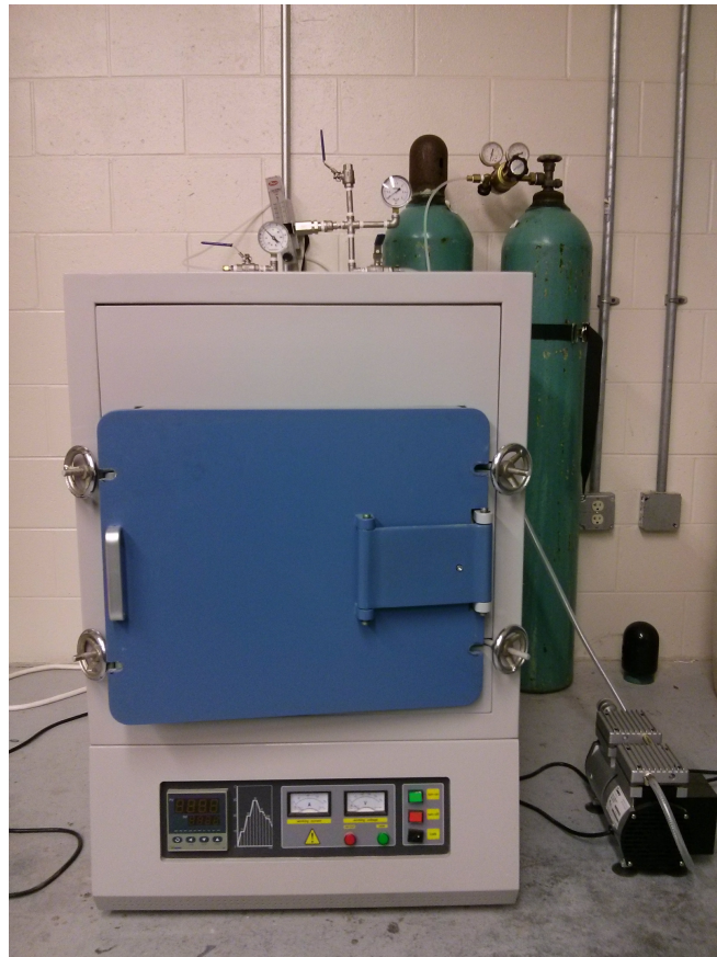
Figure 3.1: Furnace used for desizing
