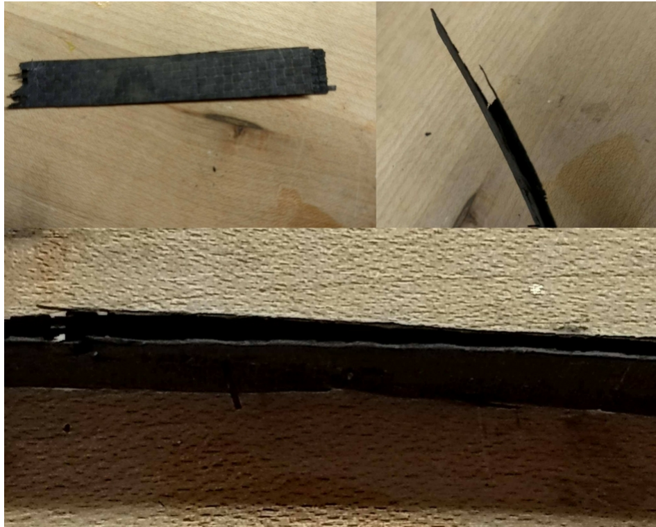
Figure 4.3: Delamination and fracture surfaces
