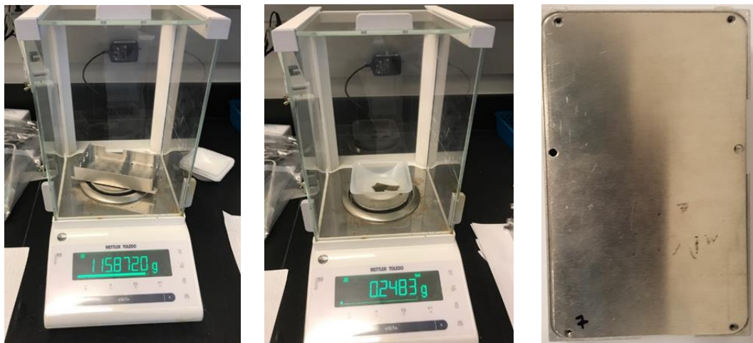
Figure 6.6 (a) Weighing of boat (b) weighing of test specimen (c) housing covered with lid.
