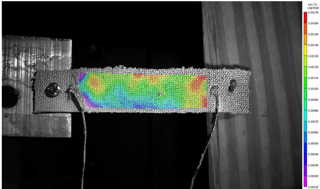
Figure 3.12. Strain map of the specimen at the maximum tension
