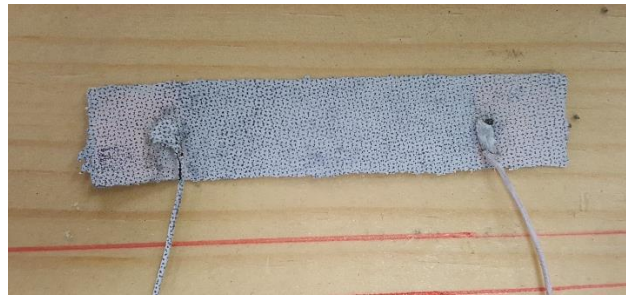
Figure 2.12. Speckled test specimen for digital image correlation
