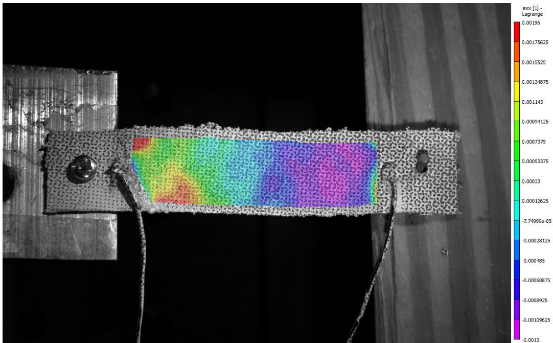
Figure 3.13. Strain map of the specimen at maximum compression
