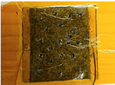
Figure 5.9. 2.5 in \times 2.5 in nanocomposites made of covered with Kapton and twenty \Phi 3mm holes are successively added.
