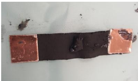
Figure 6.2 Tearing of layers of buckypaper due to application of 3M 2216 B/A gray epoxy
