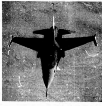
This view of the AFTI/F-16 from a KC-135 aerial tanker aircraft shows the Forward Looking Infrared (FLIR) pod on the right wing, and a dummy aerodynamic load on the left.
