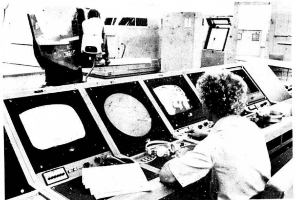
A student monitors the "Anytown USA" radar screen. (Right) Anytown is like most aviation oriented towns in America in that it has six VOR's, four NDB's, and two ILS approaches. The control console has a television monitoring system which allows instructors to monitor their students while acting as air traffic controller. The center controller can simultaneously operate, monitor, introduce malfunctions, and act as air traffic controller for all four GAT's. Riddle is also using a general medium size transport simulator which has a cockpit similar to the Convair 440.
