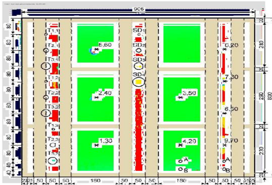
Figure C5. NDI C-Scan image of honeycomb composite panel BVID testing data. Reproduced from “Aerospace Applications,” by T. Marshall, Sonatest, Ltd., n.d., NDT Inspection of Composites for In-Service Defects , p. 31.
