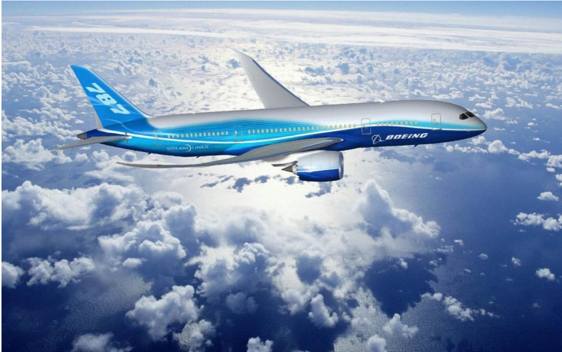
Figure B2. Illustration of Boeing 787 Dreamliner showing blended wing tips. Reproduced from the Boeing website. Copyright © 2013 by the Boeing Company. Reprinted with permission.
