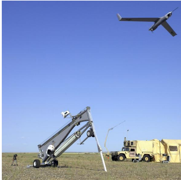
Figure 1. Scan Eagle UAS. Public domain image obtained from http://www.af.mil/About-Us/Fact-Sheets/Display/Article/104532/scan-eagle/ . The Scan Eagle UAS typically operates under 15,000 feet, and sports a 5-foot long fuselage with a wingspan of 10 feet. Reference platform details at: http://www.boeing.com/history/products/scaneagle-unmanned-aerial-vehicle.page
