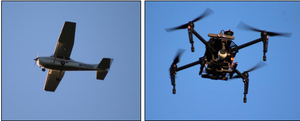
Figure 2. [LEFT] G-1000 equipped, Cessna 172/S aircraft (36-ft wingspan) used during the experiment. [RIGHT] DJI Matrice 100 (27-in width, rotor hub-to-rotor hub) outfitted with 50mAh STROBON Navigation Strobe Lights affixed to UAS anterior surface. STROBON technical information available from: http://www.flytron.com/led-systems/150-strobon-navigation-strobe-blue.html
