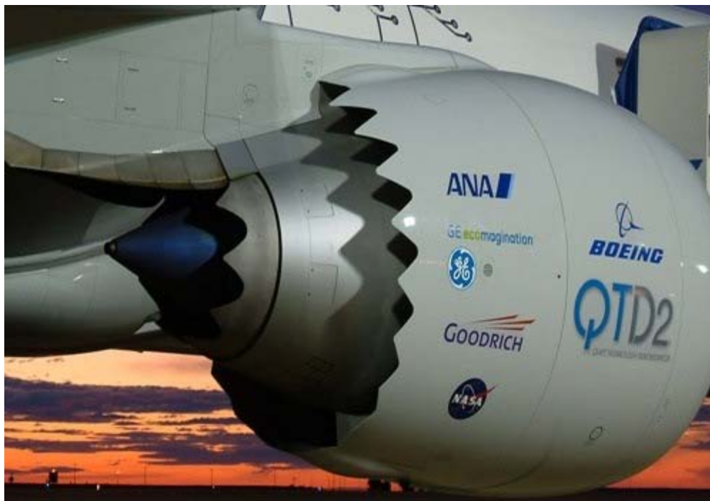
Figure 2.9. Turbofan engine with chevrons
