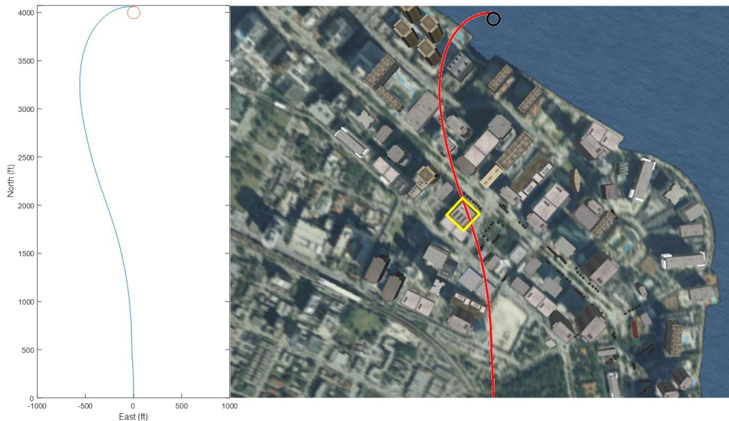
Figure 63: UAV path for complex urban virtual reality scenario
