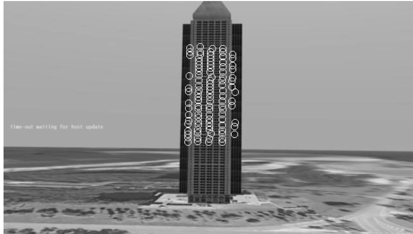
Figure 55: Feature point overlay of UAV camera view for single building avoidance
