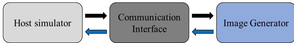
Figure 52: process overview for Pro-Nav guidance virtual reality integration
