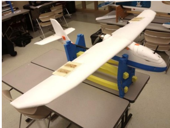
Figure 6.1. Skywalker 1880 Assembled RC Model with MFC Halved-Ailerons
