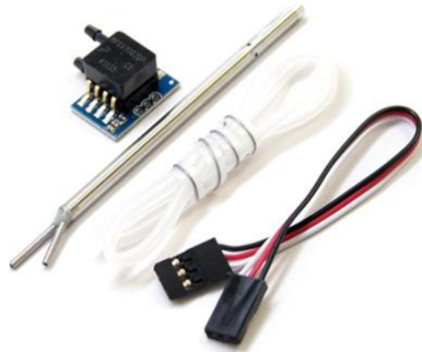
Figure 6.7. Pitot Tube and Pressure Sensor
