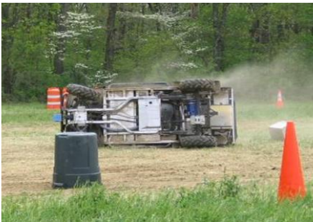
Fig. 1: Rollover of large mobile robot due to an attempted maneuver beyond the vehicle's dynamic limits.
