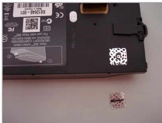
Image 24: Removing Microsoft sticker reveals the fourth screw and indicates the drive has been accessed
