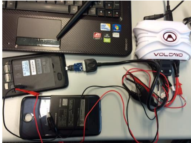
Picture 1. Cable connection using Volcano Box
