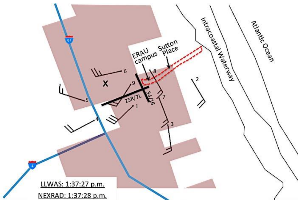
Figure 4. Local analysis over Daytona Airport and vicinity about 30–60 seconds before tornado touchdown just east of intersection of runways 25R/7L and 34/16. Path of tornado outlined in dashed red line with locations of ERAU campus and Sutton Place Apartments as shown. LLWAS winds plotted for closest time to NEXRAD scan. Tower numbers are indicated in black. Maximum base reflectivities from NEXRAD (~50 dBZ and greater) are shown by shaded area. The X denotes the location of a NEXRAD-identified circulation about 2 km above ground.
