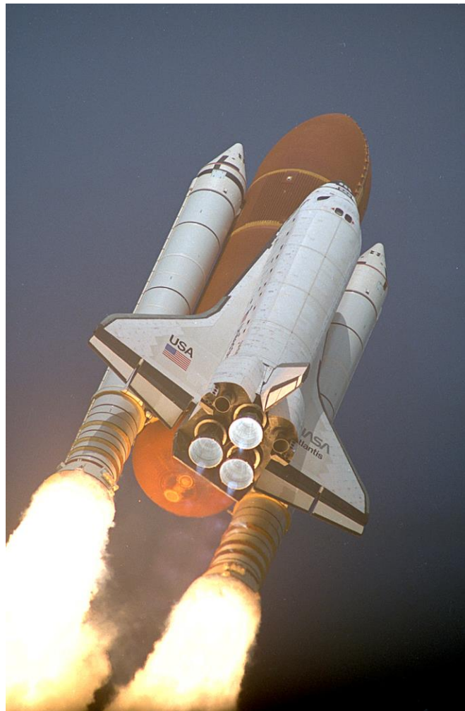
Figure 1. After roll maneuver and short vertical ascent, the mighty STS Space Shuttle starts a gravity turn (GT). In addition to three main engines, the two OMS engines are also clearly visible. Image courtesy of NASA/Marshall Space Flight center (NASA-MSFC).
