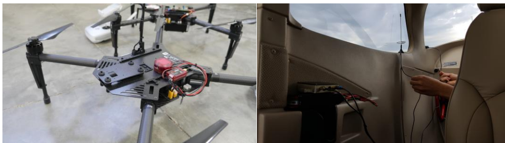
Figure 2. uAvionix proprietary ADS-B device installed on UAS (left) and aircraft (right). (Used with permission)
