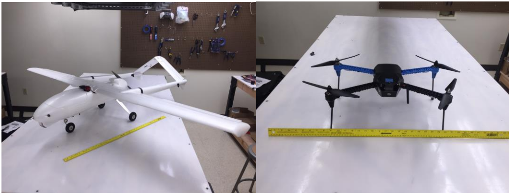
Figure 1. Anaconda Fixed-Wing UAS (left). Iris Quadcopter UAS (right). During the experiment, the Iris was colored white to increase visibility.
