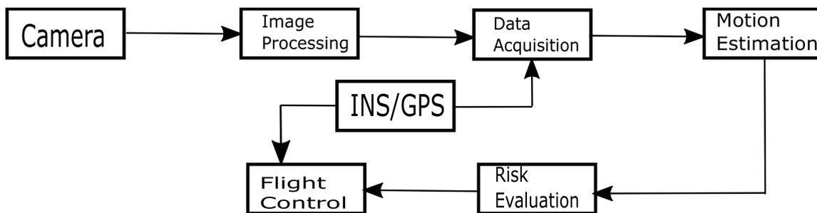
Figure 1.1. Diagram of the vision-based sense and avoid system.
