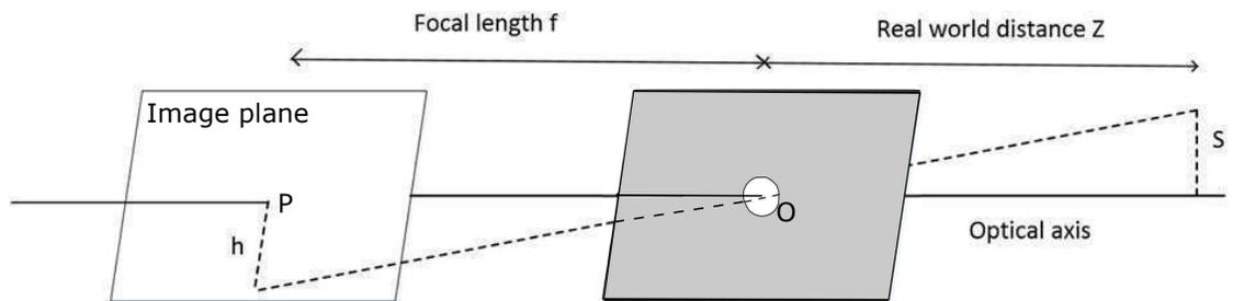
Figure 2.1. Pinhole camera model.
