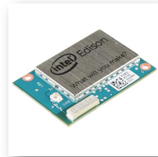
Figure 2: Intel Edison Board
