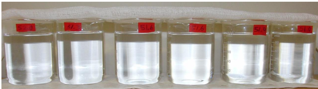
Figure 2.3 Solutions covered with muslin gauze for natural evaporation test.
