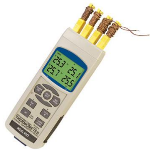
Figure 2.9 Omega 4-Channel Portable Thermometer/ Data Logger used in study.
