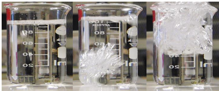
Figure B.2 Violent vapor release sequence of subcooled boiling 1000 PPM SLS solution.
