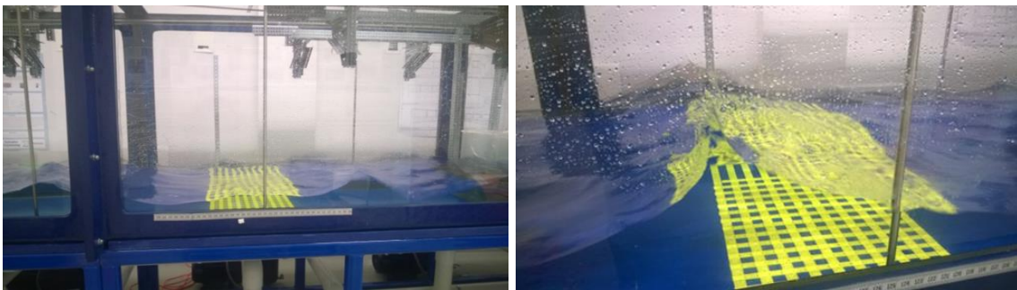
Figure 23: Grid placement inside the tank
